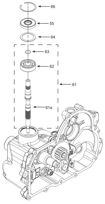
Figure 18, Input Shaft
