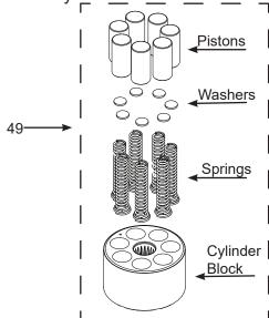
Figure 20, Pump Block Assembly
