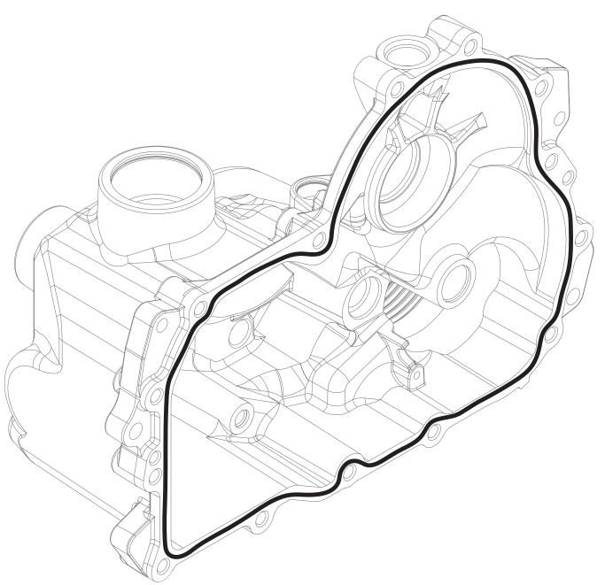
Figure 31, Sealant Application Diagram
