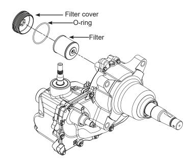
Figure 3a, Filter Components
