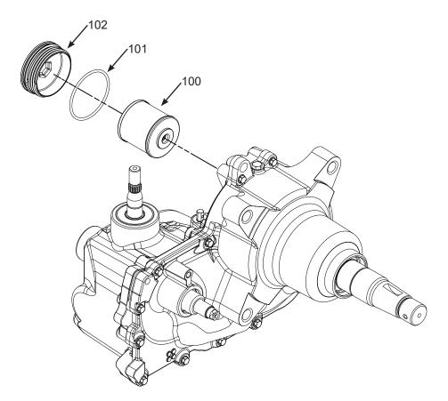
Figure 11, Filter and Filter Cover
