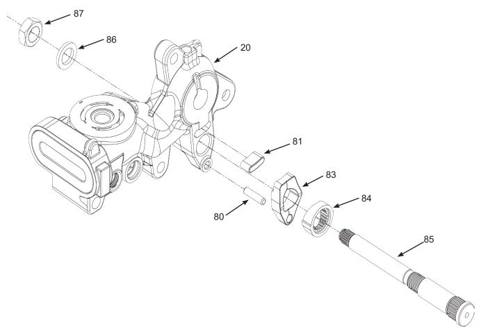
Figure 25, Brake Assembly
