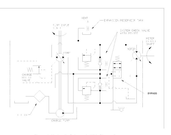
Figure 1, Hydraulic Schematic With Charge Pump
