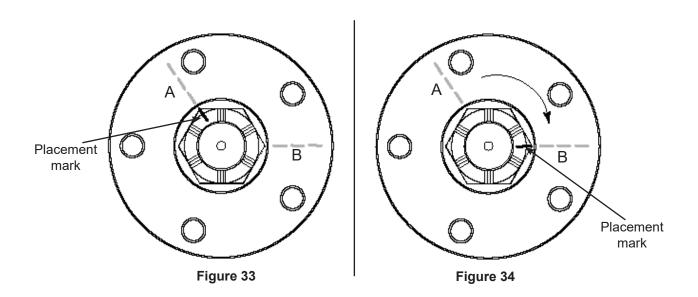
Figure 33 / Figure 34, Alternate Torque Method
