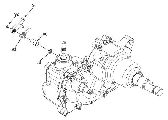
Figure 12, Brake Assembly
