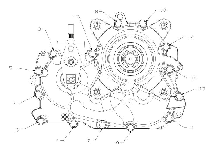
Figure 32, Screw tightening sequence
