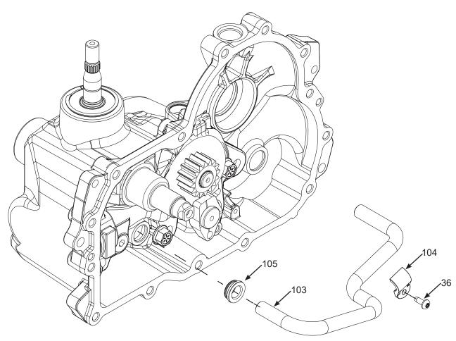
Figure 18, Filter Tube
