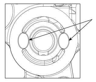
Figure 29, Motor Block Running Surface
