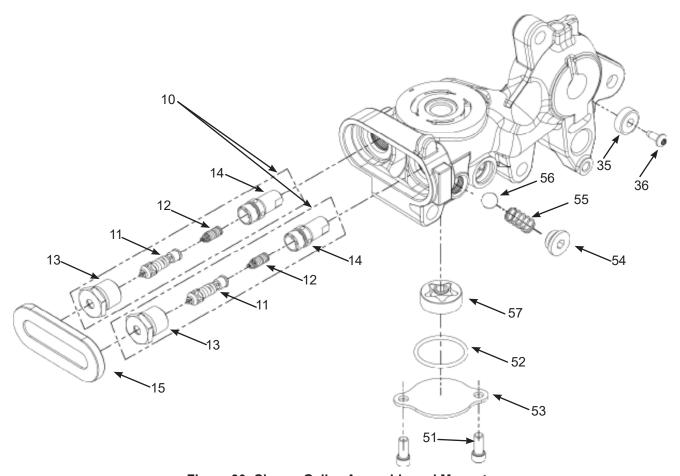
Figure 30, Charge Galley Assembly and Magnet
