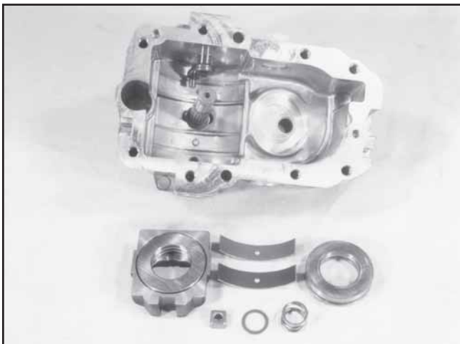
Swashplate, Cradle Bearings, Block Spring and Washer Removed
