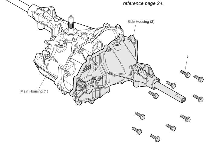
Figure 15, Side Housing Removal
