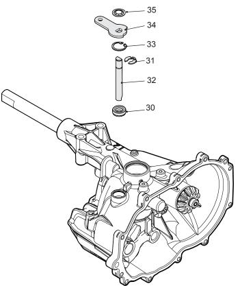
Figure 25, Bypass Arm and Rod
