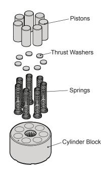
Figure 28, Pump/Motor Cylinder Block Assembly
