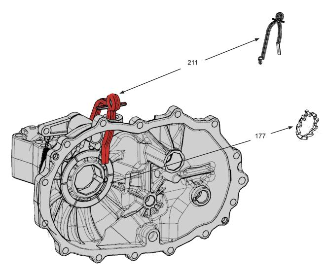
Figure 18, Differential Lock Cam Clamp
