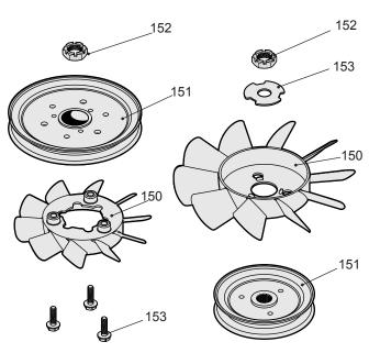
Figure 8, Fan and pulley configuration
