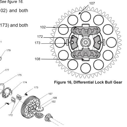
Figure 17, Differential Lock Assembly
