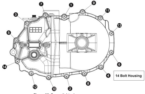
Figure 32, Screw tightening sequence
