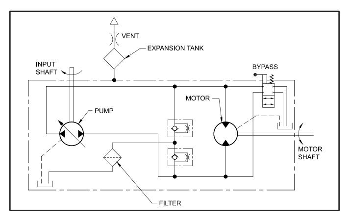
Figure 1, T2 Hydraulic Schematic
