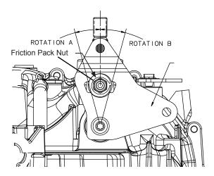
Figure 6, Friction Pack Adjustment
