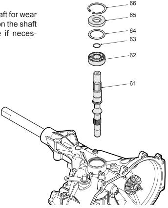
Figure 22, Input Shaft
