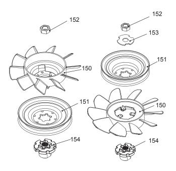
Figure 9, Hub, fan and pulley configuration
