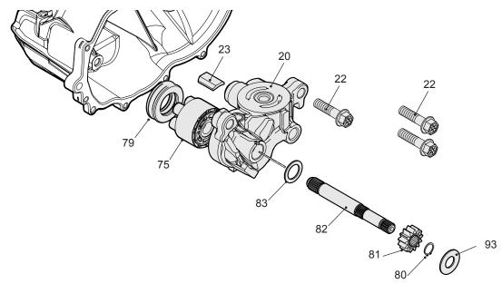
Figure 26, Center Section, Motor Shaft & Motor Block
