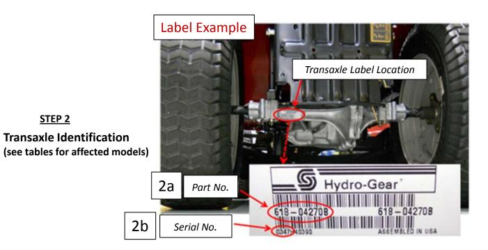
Step 1. Identify the mower Step 2. Identify the transaxle
